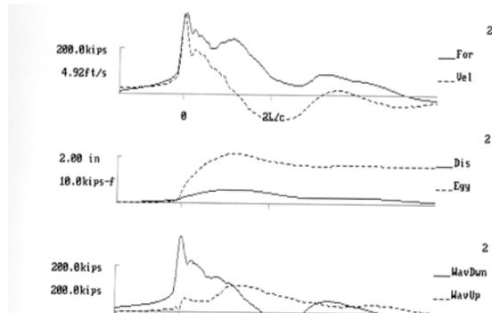
Fig. 19 Wave traces from Pile T3 at BOR
