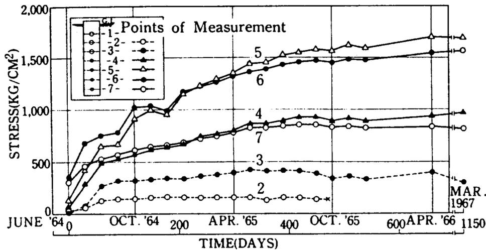
Fig. 7. Shortening of Pile cE<sub>43</sub> measured during June 1964 through March 1967 (Endo et al., 1969)
