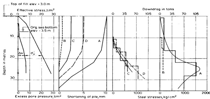
Fig. 2. Distribution of soil stress, excess pore pressure, shortening of piles, and load distribution (Bjerrum et al., 1969)
