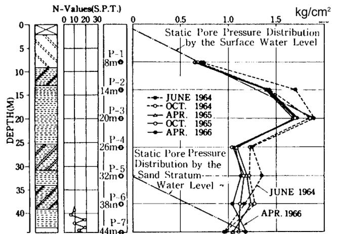
Fig. 6. Pore pressure profile at the test site (Endo et al., 1969)
