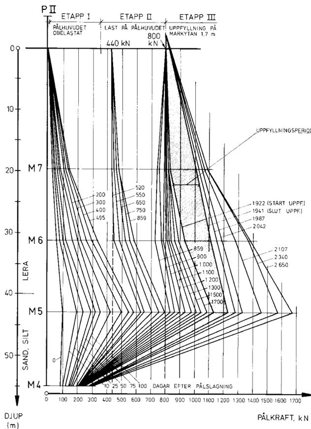
Fig. 12 Vertical distribution of load in Pile II (Bjerin, 1977)
