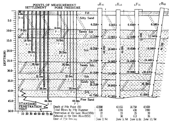
Fig. 4. Vertical view of test site and piles (Endo et al., 1969)
