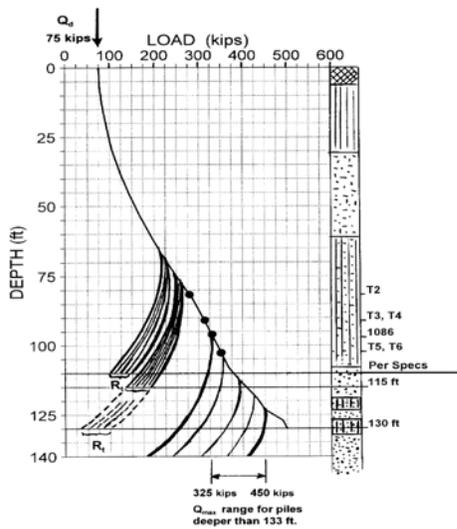
Fig. 23 Long-term Load Distribution per Final Design
