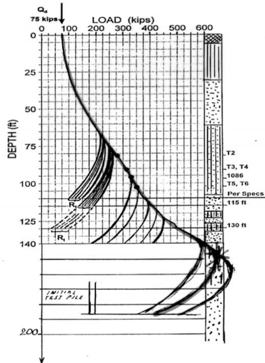
Fig. 24 Long-term Load Distribution per Initial Design
