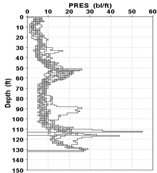
Fig. 25 Driving diagram (ten construction piles)
