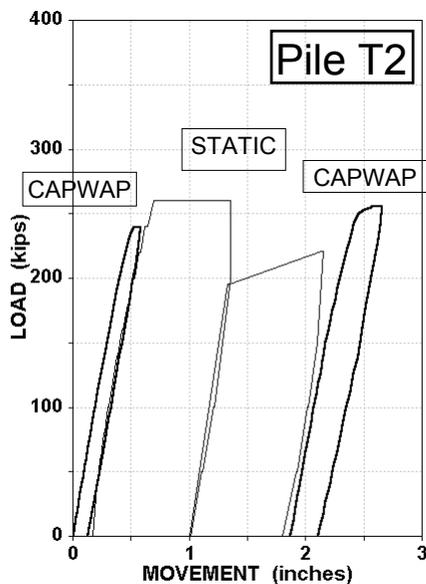
Fig. 20 Test Pile T2. Static tests and CAPWAP simulated static test
