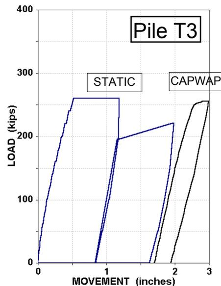
Fig. 21 Test Pile T3. Static tests and CAPWAP simulated static test
