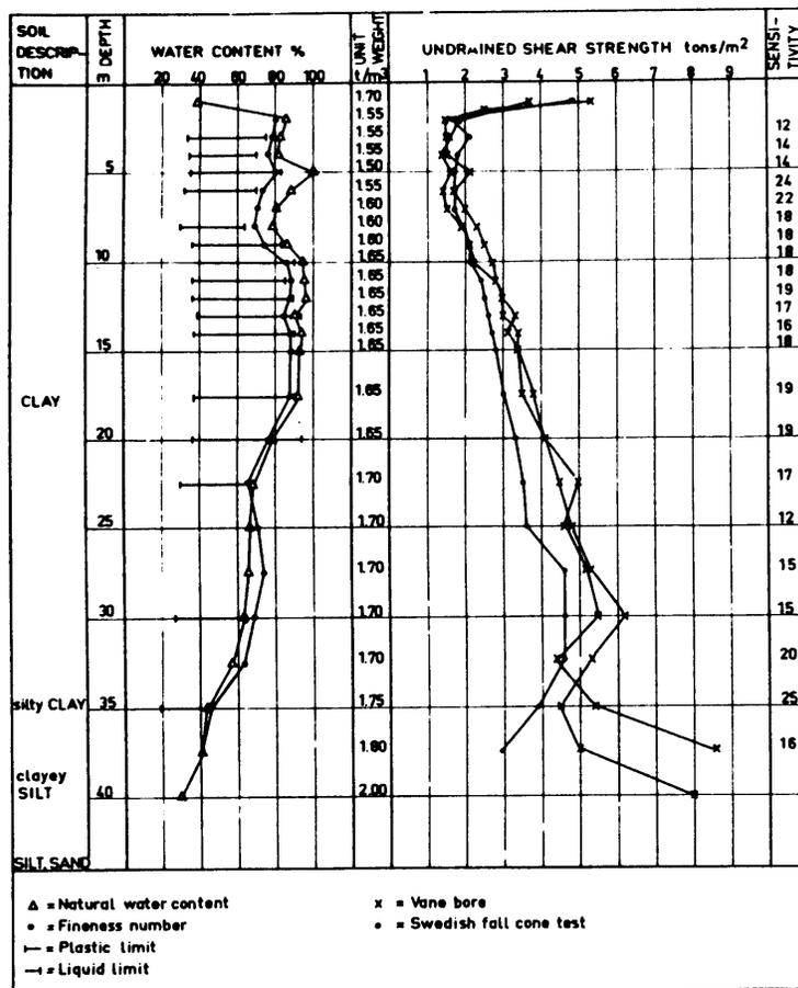
Fig. 10. Soil profile at the Bäckebo site (Fellenius 1972)
