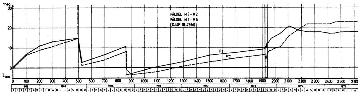
Fig. 14 Average shaft shear in Piles PI and PII between Load Cells M2 and M3, and M6 and M7 (Bjerin, 1977)
