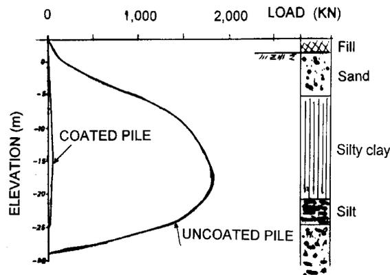
Fig. 15 Load distribution on two pipe piles, one bitumen-coated and one uncoated (Walker et al., 1973)
