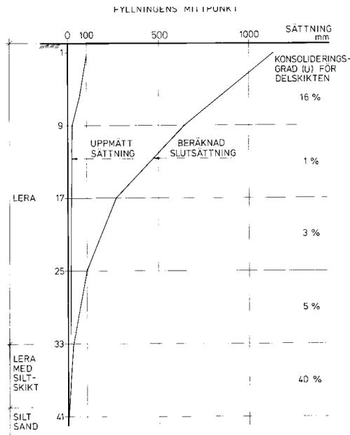
Fig. 13 Vertical distribution of measured and calculated consolidation settlement (Bjerin, 1977)
