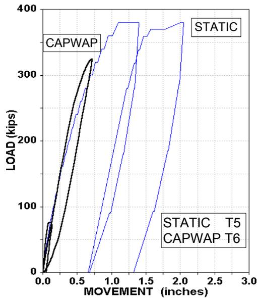
Fig. 22 Test Pile T5 Static tests and T6 CAPWAP simulated static test
