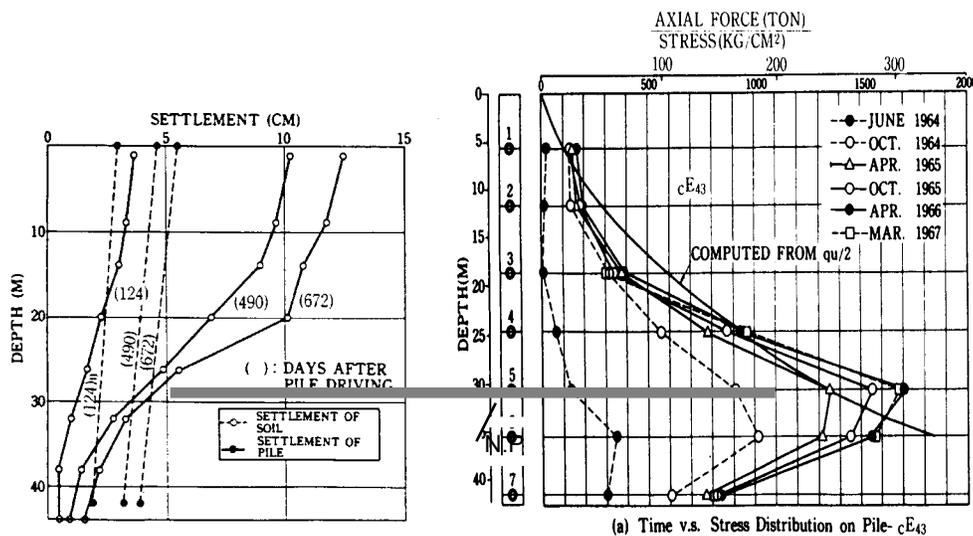
Fig. 9. Distribution of settlement of the soil and Pile cE43 and load distribution in Pile cE43 (Endo et al., 1969)
