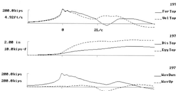
Fig. 18 Wave traces from Pile T3 at EOID
